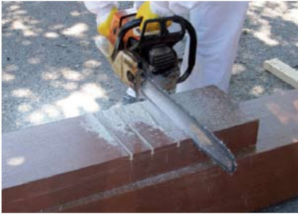
Left: FFU sleepers can be cut using the same hand-held tools as wood.
